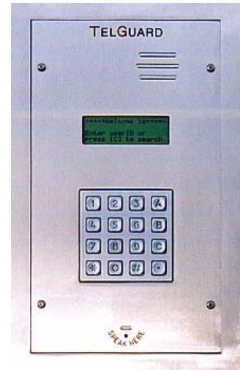
PSTN / PABX Telephone based entry phones
